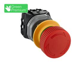
Harmony XB5, Emergency stop, plastic, red mushroom Ø40, Ø22, trigger latching turn to release, monitoring contact, 1 NO + 2 NC
