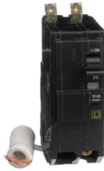
Mini circuit breaker, QO, 20A, 2 pole, 120/240VAC, 10kA, bolt on, 30mA grd fault B
