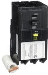
Mini circuit breaker, QO, 50A, 3 pole, 208Y/120VAC, 10kA, plug in, 6mA grd fault A, pigtail
