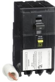
[TAA] Mini circuit breaker, QO, 30A, 3 pole, 208Y/120VAC, 10kA, plug in, 6mA grd fault A, pigtail
