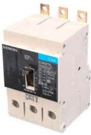
SIEMENS LOW VOLTAGE PANELBOARD MOUNT G FRAME CIRCUIT BREAKER WITH THERMAL - MAGNETIC TRIP UNIT. UL LISTED NGB FRAME WITH STANDARD BREAKING CAPACITY. 110A 3-POLE (14KAIC AT 600Y/347V) (25KAIC AT 480Y/277V). SPECIAL FEATURES: LOAD SIDE LUGS ONLY (TC1GG20) WIRE RANGE: 8 - 1/0 AWS (CU/AL). DIMENSIONS (W x H x D) IN: 3 x 5.4 x 2.8.
