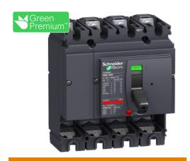
Circuit breaker basic frame, ComPact NSX160N, 50kA at 415VAC 50/60 Hz, 160A, without trip unit, 4 poles
