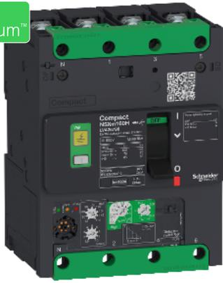
circuit breaker ComPact NSXm F (36 kA at 415 VAC), 4P 4d, 100 A rating Micrologic 4.1 trip unit, lugs and busbar connectors
