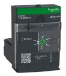
Advanced control unit, TeSys Ultra, 4.5A to 18A, 3P motors, protection & diagnostic, class 10, coil 110-240VAC/DC
