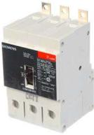
SIEMENS LOW VOLTAGE PANELBOARD MOUNT G FRAME CIRCUIT BREAKER WITH THERMAL - MAGNETIC TRIP UNIT. UL LISTED LGB FRAME WITH VERY HIGH BREAKING CAPACITY, 90A 3-POLE (14KAIC AT 600Y/347V) (65KAIC AT 480Y/277V). SPECIAL FEATURES: LOAD SIDE LUGS ONLY (TC1GG20) WIRE RANGE: 8 - 1/0 AWS (CU/AL). DIMENSIONS (W x H x D) IN: 3 x 5.4 x 2.8.
