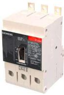
SIEMENS LOW VOLTAGE PANELBOARD MOUNT G FRAME CIRCUIT BREAKER WITH THERMAL - MAGNETIC TRIP UNIT. UL LISTED LGB FRAME WITH VERY HIGH BREAKING CAPACITY. 80A 3-POLE (14KAIC AT 600Y/347V) (65KAIC AT 480Y/277V). SPECIAL FEATURES: LOAD SIDE LUGS ONLY (TC1GG20) WIRE RANGE: 8 - 1/0 AWS (CU/AL). DIMENSIONS (W x H x D) IN: 3 x 5.4 x 2.8.
