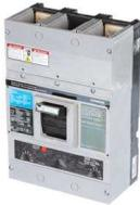
SIEMENS LOW VOLTAGE SENTRON MOLDED CASE CIRCUIT BREAKER WITH THERMAL - MAGNETIC TRIP UNIT, STANDARD 40 DEG C BREAKER JD FRAME WITH STANDARD BREAKING CAPACITY AND NON INTERCHANGEABLE TRIP. MEETS UL 489 / IEC 60947-2 STANDARDS. 350A 2-POLE BREAKER (65KAIC AT 240V). SPECIAL FEATURES: NO LUGS INSTALLED. DIMENSIONS (W x H x D) IN: 7.5 x 11 x 4.
