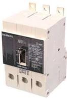
SIEMENS LOW VOLTAGE PANELBOARD MOUNT G FRAME CIRCUIT BREAKER WITH THERMAL - MAGNETIC TRIP UNIT. UL LISTED HGB FRAME WITH HIGH BREAKING CAPACITY. 80A 3-POLE (14KAIC AT 600Y/347V) (35KAIC AT 480Y/277V). SPECIAL FEATURES: LOAD SIDE LUGS ONLY (TC1GG20) WIRE RANGE: 8 - 1/0 AWS (CU/AL). DIMENSIONS (W x H x D) IN: 3 x 5.4 x 2.8.
