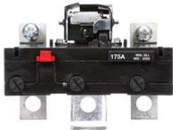
SIEMENS LOW VOLTAGE SENTRON MOLDED CASE CIRCUIT BREAKER WITH THERMAL - MAGNETIC TRIP UNIT. TRIP UNIT FOR FD FRAME WITH STANDARD BREAKING CAPACITY, MEETS UL 489 / IEC 60947-2 STANDARDS. 175A 3-POLE BREAKER (22KAIC AT 600V) (35KAIC AT 480V). SPECIAL FEATURES: LINE AND LOAD SIDE LUGS (TA1FD350A) WIRE RANGE: 6AWG - 350KCM (CU) / 4AWG - 350KCM (AL). DIMENSIONS (W x H x D) IN: 4.5 x 9.5 x 4.
