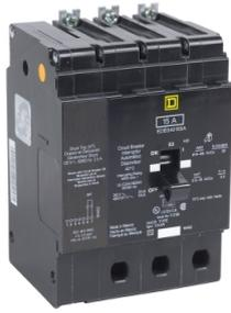
[TAA] Mini circuit breaker, E-Frame, 20A, 3 pole, 480Y/277VAC, 65kA max, bolt on, shunt trip
