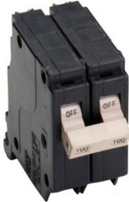
Eaton CH Thermal magnetic circuit breaker, Type CH 3/4-Inch standard circuit breaker, 100 A, 10 kAIC, Two-pole, 120/240V, CH, Common breaker trip, 14AWG – 1/0AWG, u/Al, CH, Type CH Loadcenters
