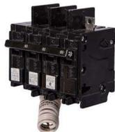
Siemens Low Voltage Molded Case Circuit Breakers General Purpose MCCBs are Circuit Protection Molded Case Circuit Breakers. 3-Pole Common-Trip circuit breaker type BQ. Rated 240V (030A) (AIR 10 kA). Special features: 120VAC Shunt Trip. Note: Load side lugs are included.
