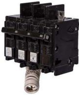
Siemens Low Voltage Molded Case Circuit Breakers General Purpose MCCBs are Circuit Protection Molded Case Circuit Breakers. 3-Pole Common-Trip circuit breaker type BQ. Rated 240V (020A) (AIR 10 kA). Special features: 120VAC Shunt Trip. Note: Load side lugs are included.
