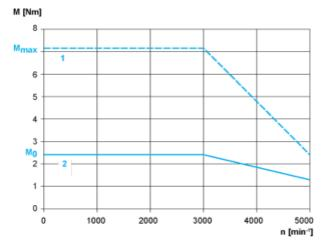
1: Peak torque2: Continuous torque
