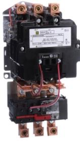
NEMA motor starter, Type S, nonreversing, Size 4, 135A, 100HP at 460VAC, up to 100kA SCCR, 3 phase, 3 pole, Motor Logic, 120VAC coil, open
