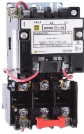
NEMA motor starter, Type S, nonreversing, Size 0, 18A, 5HP at 460VAC, 5kA SCCR, 3 phase, 3 pole, melting alloy, 480VAC coil, open
