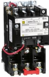
[TAA] NEMA motor starter, Type S, nonreversing, Size 0, 18A, 5HP at 460VAC, 5kA SCCR, 3 phase, 3 pole, melting alloy, 120VAC coil, open
