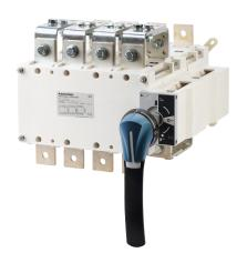
SIRCOVER Bypass provide on-load transfer between two sources for any low voltage power circuit, as well as safety isolation by double breaking per pole. This combination of three interlocked load break switches provides bypass to an UPS or other critical devices, allowing maintenance of a critical equipement while maintaining the supply of the load. There are available in 3 or 4 poles.
