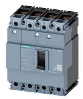
circuit breaker 3VM1 IEC frame 160 breaking capacity class S Icu=36kA @ 415V 4-pole, line protection TM210, FTFM, In=20A overload protection Ir=20A, not adjustable short-circuit protection Ii=16 x In N conductor protection 100% nut keeper kit
