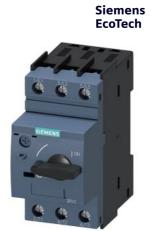
Circuit breaker size S0 for motor protection, CLASS 10 A-release 34...40 A N-release 480 A screw terminal Standard switching capacity
