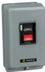
Manual starter, integral horsepower, NEMA M0, 600VAC, 2 pole, 2HP at 230VAC, 1 phase, no indicator, NEMA 1
